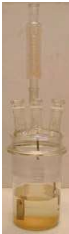
Figure 37.4.2.2: Exposure receptacle with reflux condenser
