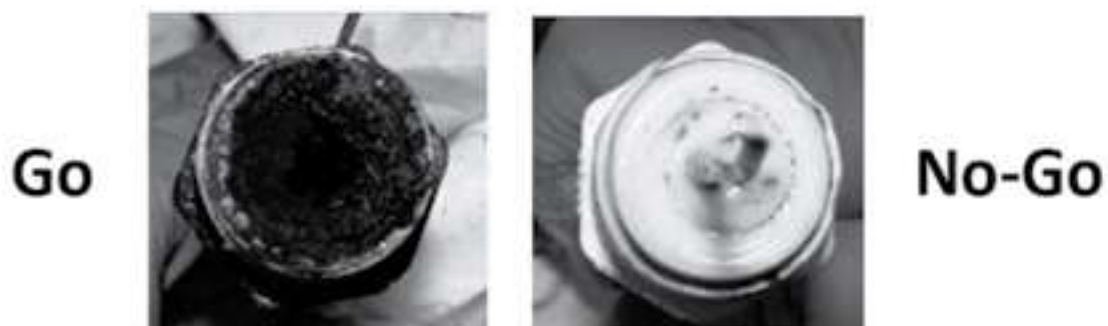
Figure 18.8.3: Typical aspect of the test cell after a "go" (left) and "no-go" (right) event
